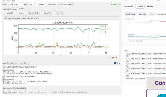
•GUI (left): One-click connect, set up LIS3DH, single-read or 1 Hz streaming, with real-time X/Y/Z plots and other
