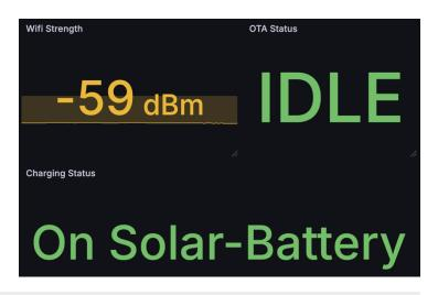
Throughput & RSSI: Walk-test across zones A to D shows RSSI is ranging from about -90 to -60 dBm and TCP throughput peaking  $\sim 4$  to 5 Mb/s with a site-wide average of 1.77 Mb/s, indicating a stable link even through partial NLOS (buildings, trees, etc...).
