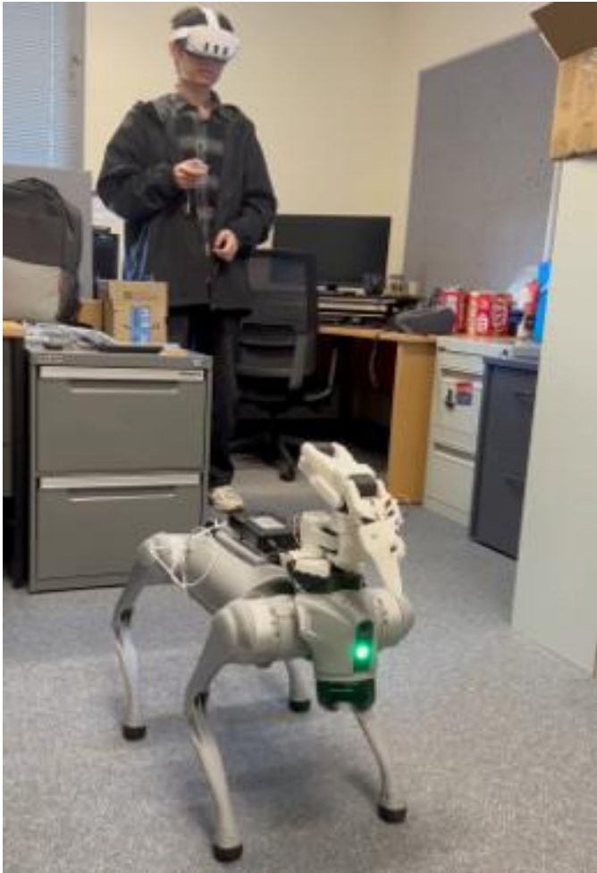
Figure 1: Loco-manipulation in practice: VR-based teleoperation of the Go2 with SO-100/101 arm in UQMM lab.
